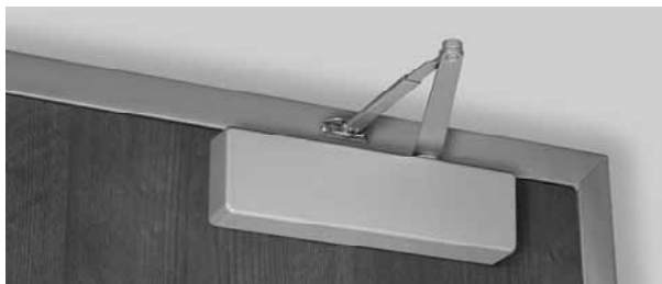
Regular Arm - Regular Arm allows closer to be installed where there is as little as 1" (25mm) of frame face or ceiling clearance.
